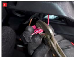
J) Use a tool such as adjustable grips or pliers to drive the metal connector into the Scotch lock to ensure good connection.
